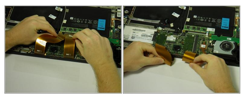
Disconnect the screen and copper colored motherboard cables and tuck them under the device to prevent future hassle.
