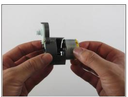
Removing these two screws will allow you to access the motor (use the same head as before)
