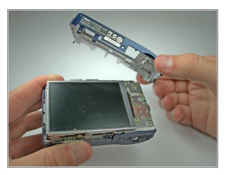
Pry the back cover from the left side of the camera. Remove the cover gently.
