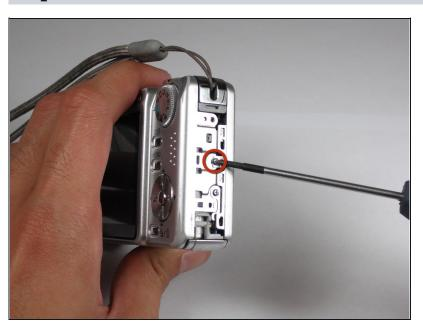
Remove the screw using a Phillips #00 screwdriver on the right side (where the caution panel used to be).
