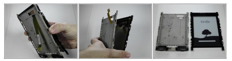
• With the clips separated, gently guide the Screen's Motherboard Connector through the hole.
