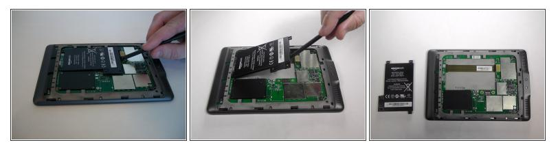
• Using the flat end of your spudger, gently pry the battery up and remove it.
