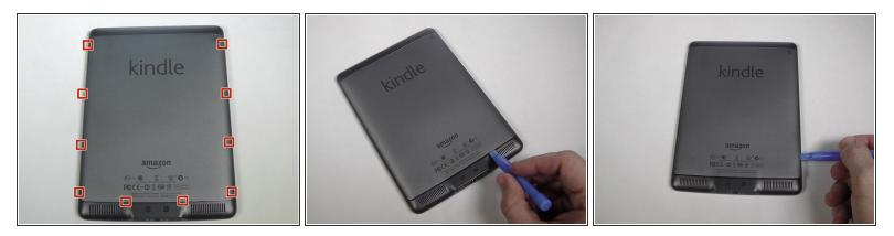
• Use the plastic opening tool to undo the ten plastic clips around the back panel of the Kindle.
