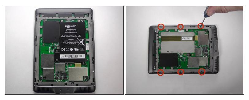
Using a Phillips #00 screwdriver, remove the six 4 mm screws to access the front plate.
