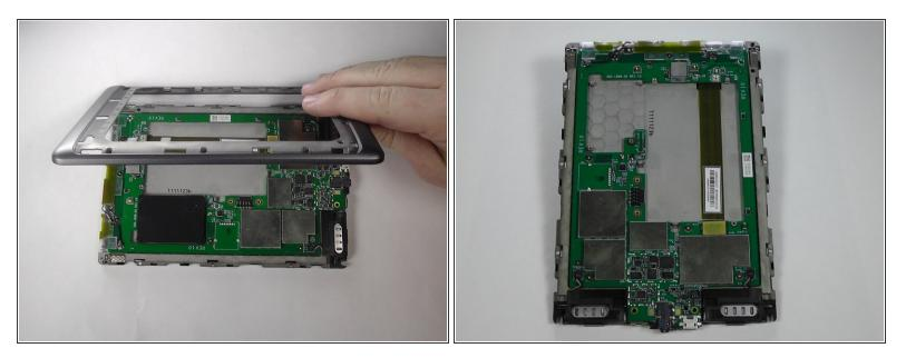
• With the screws removed, gently remove the case from the internals.
