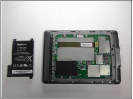
Using the flat end of your spudger, gently pry the battery up and remove it.
