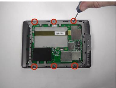
Using a Phillips #00 screwdriver, remove the six 4 mm screws to access the front plate.
