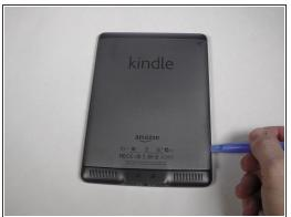
Use the plastic opening tool to undo the ten plastic clips around the back panel of the Kindle.
