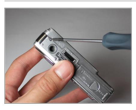
Remove the screw using the Phillips #00 screwdriver from the bottom of the camera, closest to the back cover.
