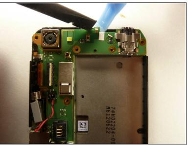
Use the spudger to push back the latch holding on the motherboard. While the latch is pushed back use the plastic opening tool to pry up the motherboard.
