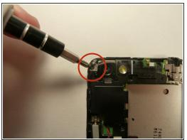
Remove the two 3.0 mm Phillips #0 screws, that are securing the camera lens.
