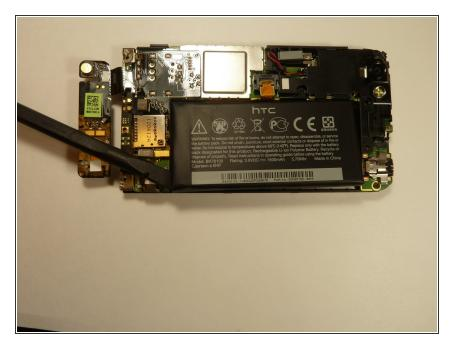
Pry up the battery with the flat end of the spudger.
