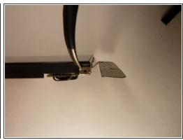
Using tweezers, pull back on the tape located on the bottom corners of the motherboard.
