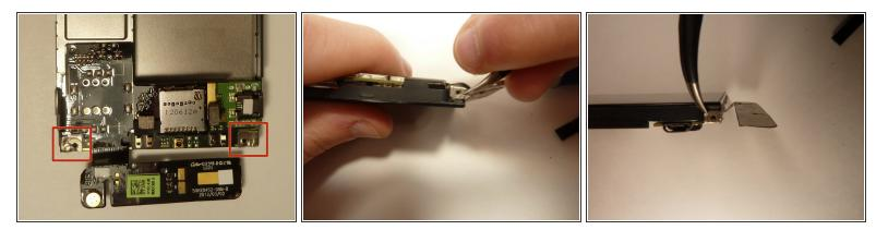
• Using tweezers, pull back on the tape located on the bottom corners of the motherboard.
