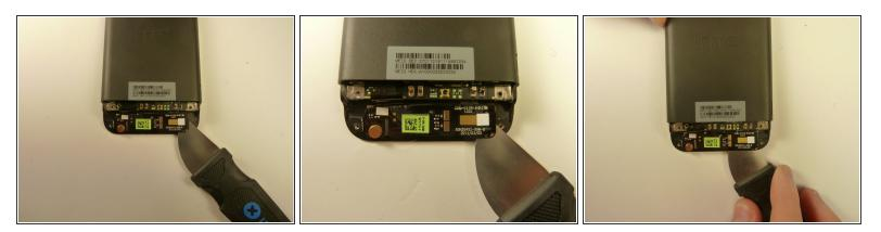
Use a Jimmy to pry up the OEM SIM and SD card reader contact.
