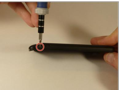
Remove the 2.0 mm Phillips #0 screws on either side of the phone.
