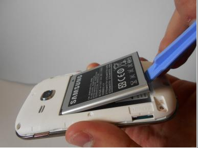
Locate the indent on the bottom left corner of the battery compartment. Use your fingers or the plastic opening tool to lift the battery from the device.
