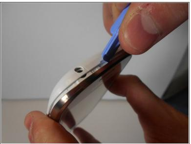
Locate the small indent in the top of the device and use your nails or the plastic opening tool to separate the cover from the mid-frame.
