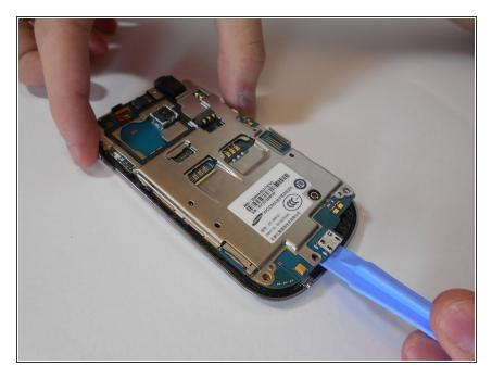
Wedge the plastic opening tool between the motherboard and front plate to dismount the motherboard and chassis from the front plate of the phone.
