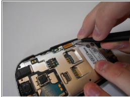
Carefully use the pointed end of the spudger to disconnect the ribbon connections on the motherboard.
