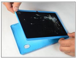
Place your Plastic Opening Tool between the screen and the case. Slowly move it around the casing while prying in a downward motion to undo the hinges holding the two together and separate the two parts.
