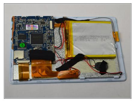
After separating the case and screen, turn your screen face down so you can see the internal parts!
