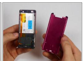
Remove the back plate from the device.
