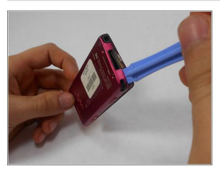
Use a plastic opening tool to loosen the bottom portion of device.
