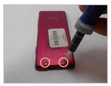
Use a Phillips #00 screwdriver to unscrew the two 5 mm screws located on the bottom of the back of the device.
