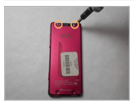
Use a Phillips #00 screwdriver to remove the two 3 mm screws located on the portion under the top panel of the device.
