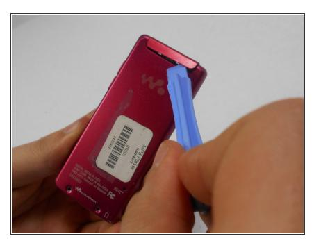
Use a plastic opening tool to loosen the top panel of the device.
