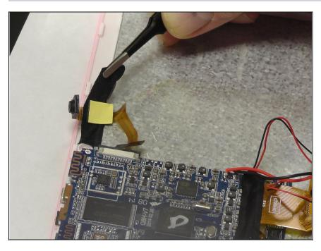
Use <u>tweezers</u> to remove the black tape holding the camera down.
