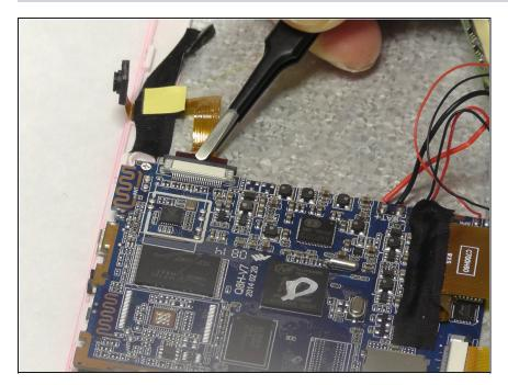
Use small needle nose pliers to carefully remove the yellow ribbon attached to the motherboard.
