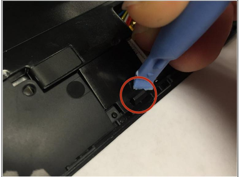
**i** The battery has one clip you will need to remove. The clip is located at the bottom right corner of the battery just above the right speaker. The speakers and wires are not secured to the battery, they may fall off.
