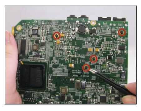
On the back side of the motherboard, use the tweezers to squeeze the four protruding clips.
