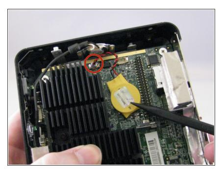
To remove the battery, pull up on the connector that is plugged into the motherboard.
