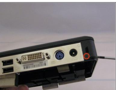
Remove the two 4mm Phillips #00 screws that are along the back of the case.
