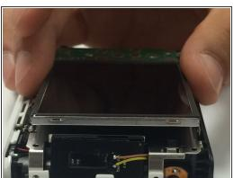
Open all the screws around the screen using Phillips #000 Screwdriver.
