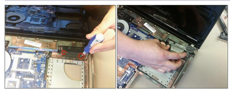
• Remove two M2.0 x 3mm flathead screws on the right side (using the small flathead screwdriver).
