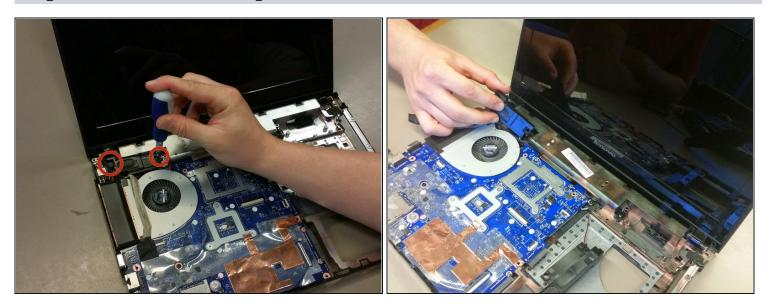
• Remove two M2.0 x <u>3mm flathead</u> screws on the left side (using the small flathead screwdriver).
