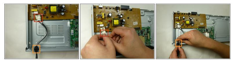
• Detach the power supply cord from the brown motherboard by pushing the locking clip on the connector, and pulling out.
