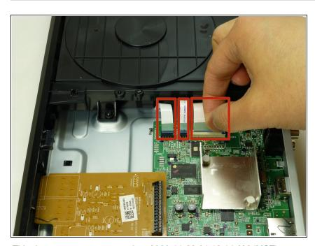
Using your fingers, pull the three tape-like cables to disconnect the disc drive from the green motherboard.
