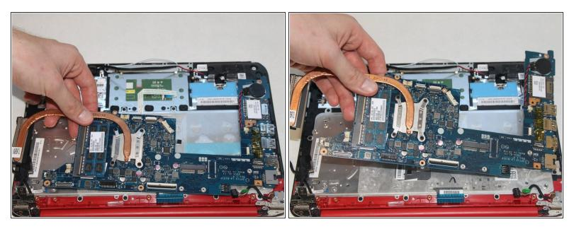
• Lift up to remove the motherboard.
