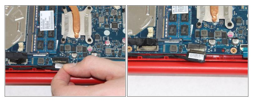
• Pull horizontally toward the hinge of the laptop to disconnect the webcam cable.
