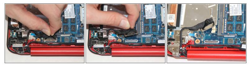
• Pull up on the black tabs to disconnect the display cable.
