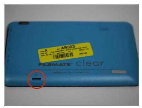
• Locate the hole on the bottom left hand side of the backplate.
