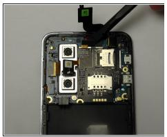
• Utilize a spudger or plastic opening tool and gently disconnect the ribbon cable that is attached to the black micro-SIM card board.
