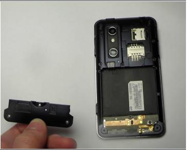
• Use your finger or opening tool to wedge the speaker out starting at the small notch at the bottom of the phone.
