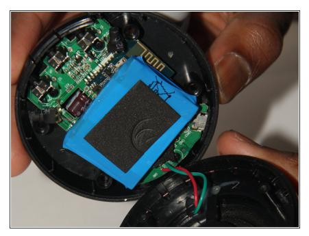
Once you've removed the screws, open the case slowly. The battery is covered in blue packaging.
