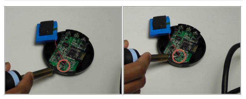
Use a solder gun to remove the battery attachments from the motherboard.
