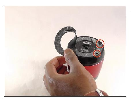
Gently remove the rubber cover to expose the screws. If necessary, poke holes through the glue residue to expose the screw heads.
