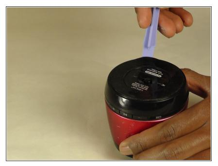
Use the plastic opening tool to pry off the rubber cover at the bottom of the speaker.
