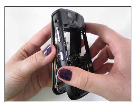
Remove the back casing by wiggling it open.
