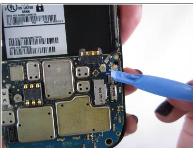
Using the small plastic opening tool, remove the side antenna cable.
