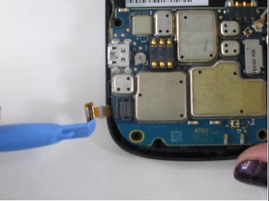
Using the small plastic opening tool, pry up the pop ribbon cable from the motherboard.
