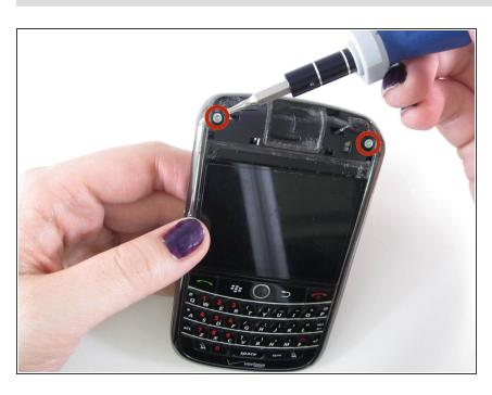
Use the T6 Torx screwdriver to remove the two 8.00mm screws from the top of the phone.
