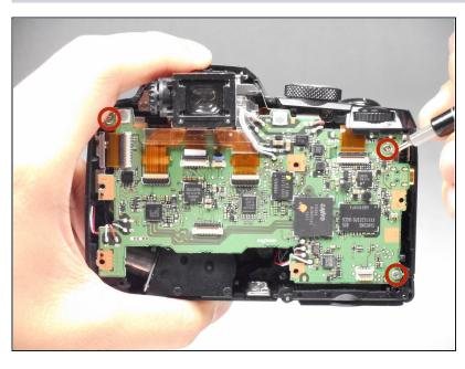
Using a Phillips #000 Precision Screwdriver, remove the three 3.0 mm screws from the motherboard.
