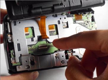
• Press your finger on the top of the latch and pull it down and towards you to open the safety latch and free the ribbon.
