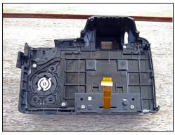
Carefully lift the back cover from the camera.
