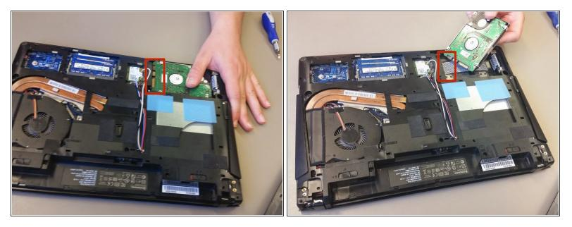
If you intend to reuse this Hard Drive/SSD, be careful with the removal. Hard impact may result in damage.
