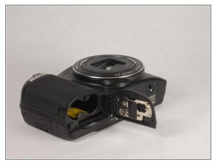
The batteries are located on the bottom of the device on the right hand side. To open the compartment press the button in and slide it towards you and pull the door open.
