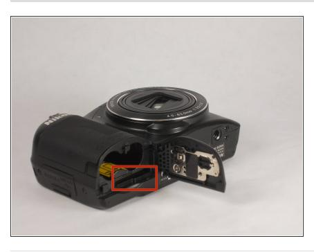
The memory card is located next to the batteries. To remove the memory card press it in and it should pop out.
