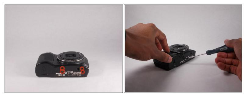
• Remove the four (3.20 mm) Phillips #00 screws at the bottom of the device.
