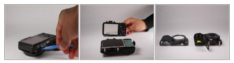
• Separate the case using the plastic prying tool. This can be done by placing the tool in the position that is shown and in the position on the left side of the camera.
