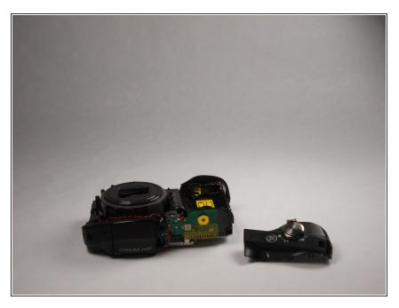
• Remove the panel containing the power and shutter button.
