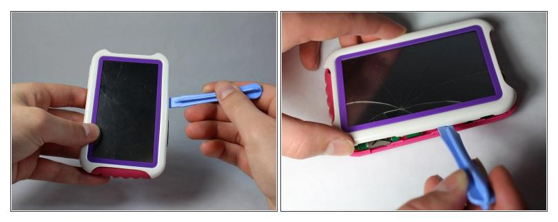
• Use the opening tool to carefully pry open the case to reveal the motherboard underneath.
