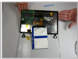
We will need to separate the battery from the panel slightly. This will allow for easier maneuverability to remove speakers. Do not separate the battery completely.
