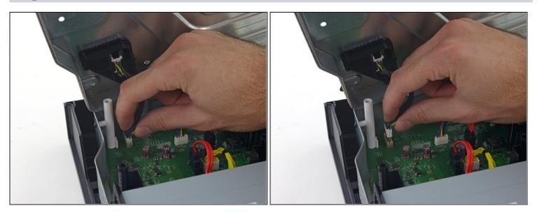
• Disconnect the Wi-Fi board interconnect cable from the motherboard.
