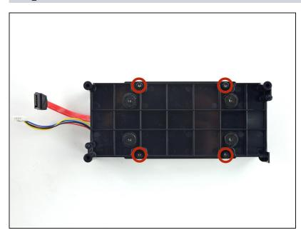
Remove the four 8.5 mm T10 Torx screws securing the hard drive assembly to the hard drive tray.
