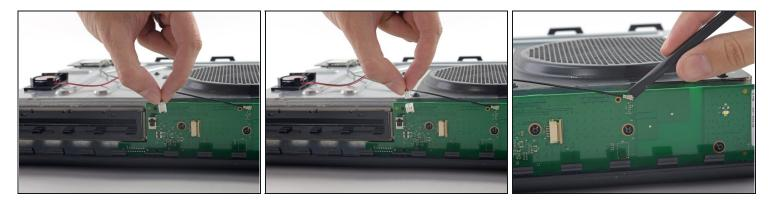
• Gently pull up on the speaker cable connector to disconnect it from the front panel board.
