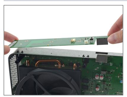
Disconnect the front panel board from its socket in the front of the motherboard.
