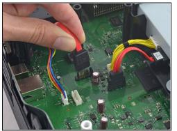
• Disconnect the hard drive SATA power and data cables from the motherboard.
