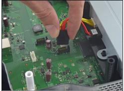
• Disconnect the optical drive power and SATA data cables from the motherboard.
