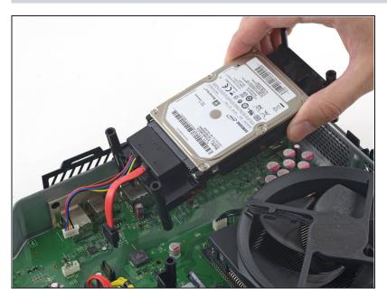
Lift and remove the hard drive tray from the Xbox.
