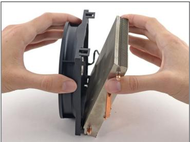
Separate the heat sink from the fan.
