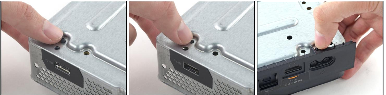
① Two small plastic plugs protrude through the rear metal case—one beneath the side USB port, and another beneath the AC in port. These plugs get caught on the lower metal case and make it hard to remove the motherboard.
