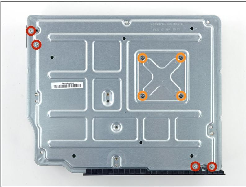
① Flip the lower metal frame and motherboard assembly over, to rest on the fan.
