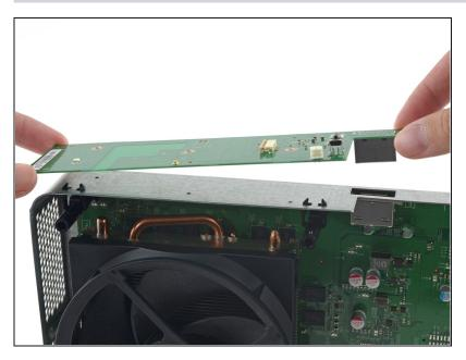
Disconnect the front panel board from its socket in the front of the motherboard.
