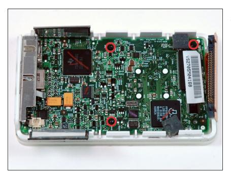
• Remove the remaining 3 T6 Torx screws from the logic board.
