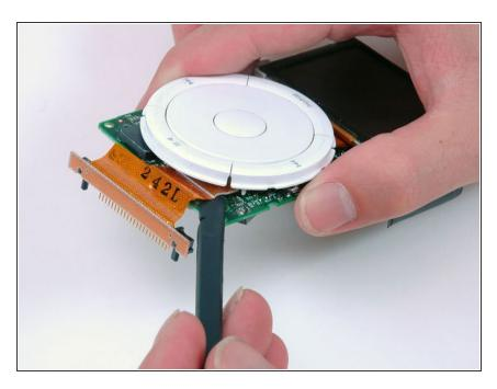
Use a spudger to carefully disconnect the orange hard drive cable from beneath the scroll wheel.
