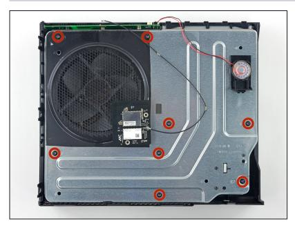
Remove the eight 65 mm Torx T10 screws from the top of the upper metal case.
