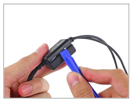
Using the plastic opening tools, pry open the cable hub.
