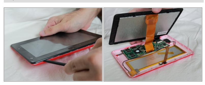
Slide the spudger along the perimeter of the device to fully separate the two pieces.
