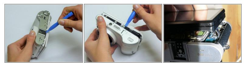
• Place a plastic opening tool into the gap between the back panel and camera body, from both the top and the bottom of camera. Carefully pry open the camera and separate the back panel.
