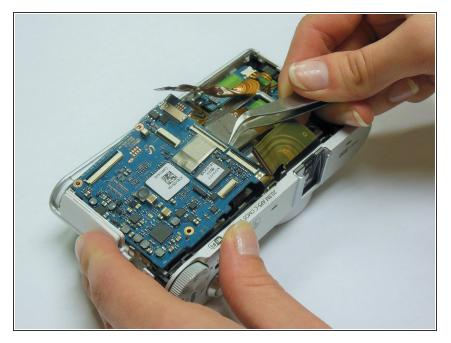
• The motherboard is now free. Pull the motherboard up and slightly away from the input compartment; it will lift out easily.
