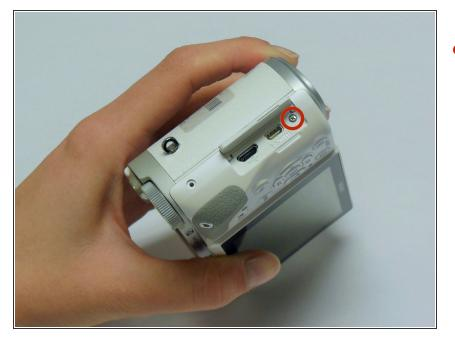
Using a Phillips #00 precision screwdriver, remove the last 4 mm screw located inside the input ports' compartment.
