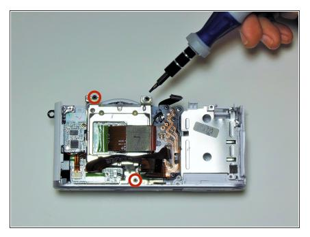
Using a 1.5mm HEX screwdriver, remove the three 5mm black screws located on the extensions of the metal housing assembly.
