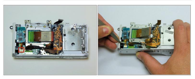
With the assistance of tweezers, pull out the last data ribbon connecting the sensor to the sound board. This ribbon must be pulled away from the board that houses the sound speaker.
