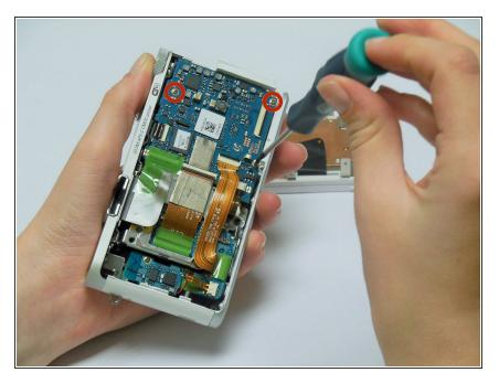
Using a Phillips #00 precision screwdriver, remove the three 4mm screws holding the motherboard in place.
