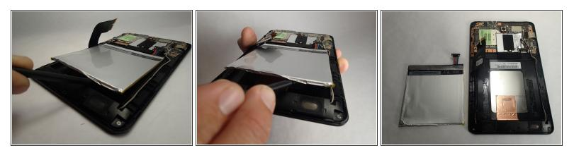
• Using a spudger carefully pry the battery up. It is glued down so slight pressure may be needed.
