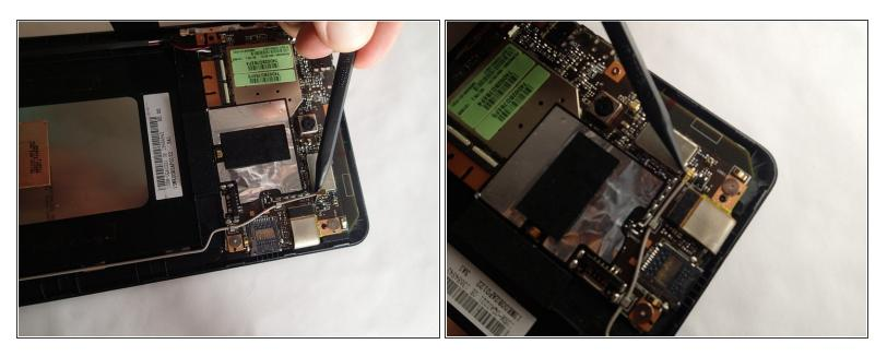
Pry the GPS Antenna cable straight up using a spudger or similar prying tool. It will be the grey
