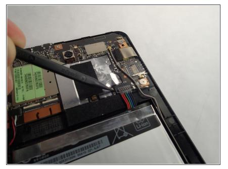
• Locate the battery connector by following the wires that come from the top right of the battery. To disconnect the battery just lift up gently on the wires. Use a spudger or blue plastic opening tool to gently lift the wires if it is hard to get a grip.
