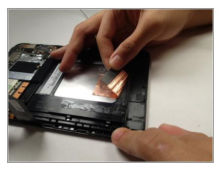
• Peel the copper tape holding the GPS Antenna down to the inside of the device using caution not to tear the tape.
