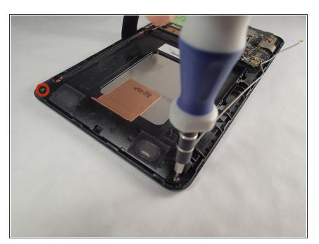
Unscrew two Philip's #000 2 mm screws located on the left and right side of the speaker housing.
