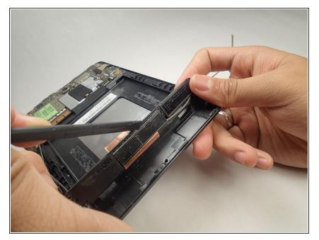
Using a spudger carefully, pry the GPS antenna from the bottom of the speaker housing.
