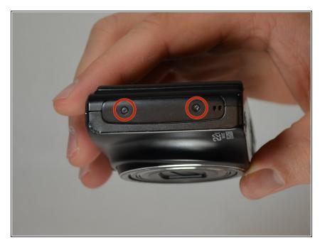
With the screen facing you, locate the two 3.5 mm screws on the left face of the camera. Remove them using a #00 Phillips screwdriver.
