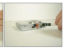
• Open the battery/memory card door and remove the 6 screws (.35cm) with a Philips 000 screwdriver. There will be two screws on the left and right sides, and two on the bottom.
