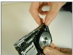
• Unscrew the .45cm screw located on the upper right corner on the back of the camera. Once the screw is off, use the spudger and unclip the piece holding the top down on the upper left on the front of the camera. It should lift off with ease.
