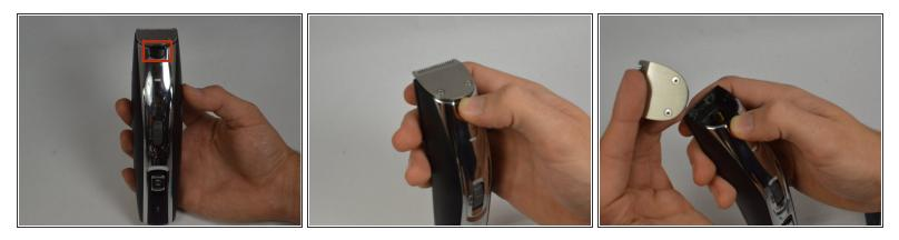
Press the black button to release the blade from its locked position.
