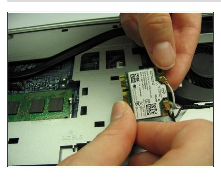
Disconnect the two antennas (one black and one white) from the wireless card.
