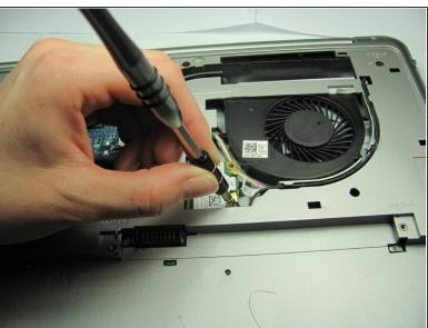
Completely unscrew the 2 mm screw that connects the WiFi card to the mother board using a Philips head screwdriver.
