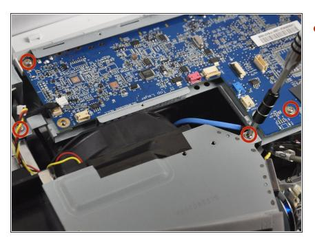
Use a Philips #1 screwdriver to remove the four 4.5 mm screws
