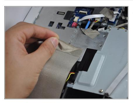
Peel off the tape that is holding the metal casing down.
