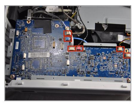
Unplug the six wires stemming from the circuit board.
