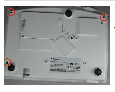
Use a Phillips #1 screwdriver to remove the three 7.5mm screws on the bottom of the device.
