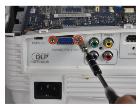
Remove the two 4.5 mm screws located on either side of the VGA/SCART port using a 5 mm nut driver. This will further release the plastic backing from the motherboard.
