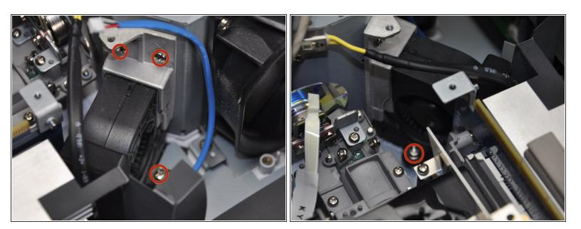
• Use a Phillips #1 screwdriver to remove four 5 mm screws. This will release the fan.
