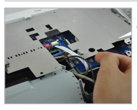
Remove the metal casing by lifting it up off of the circuit board.
