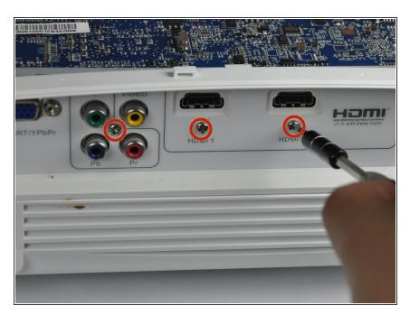
Remove the three 4.5 mm screws using the Philips #1 screwdriver.
