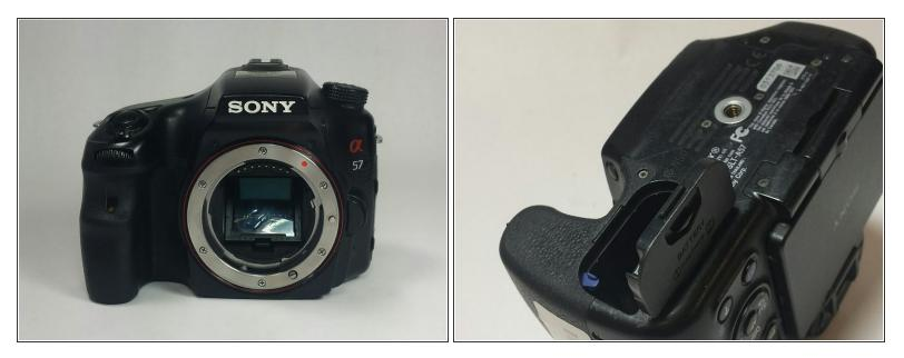
• Remove battery from compartment under camera.
