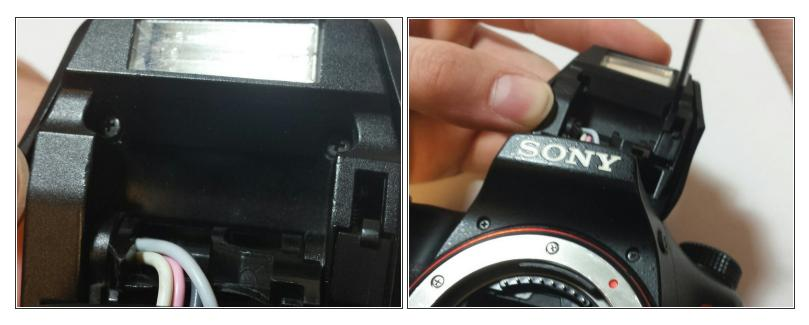
• Open the flash and unscrew the two 1.5mm screws next to the bulb on the bottom of the flash flap.
