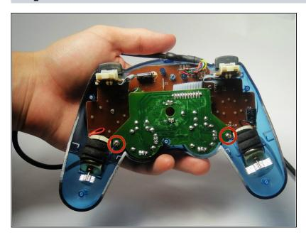
Remove the two 7 mm screws on the closest circuit board.
