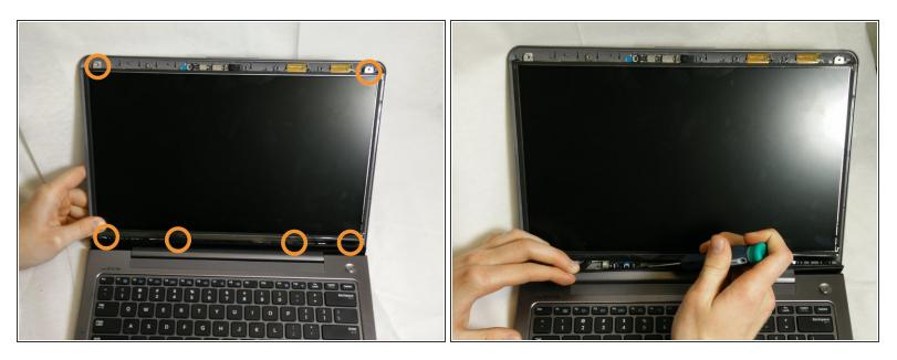
• Unscrew the six 3.7 mm screws holding the screen in place.
