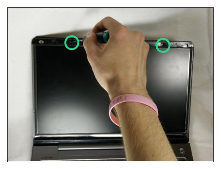
• Remove the frame by unscrewing the two 3.7 mm screws at the top.
