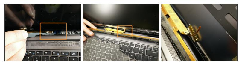
There is a small, skinny wire leading from the bottom of the touchscreen to the joint of the laptop.
