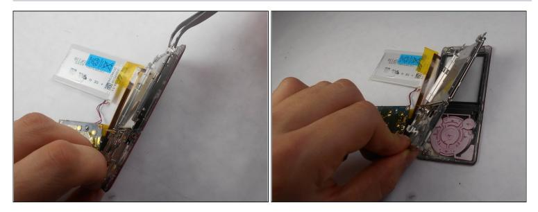
• Disconnect the metal shielding plate from the front panel with tweezers or a plastic opening tool.
