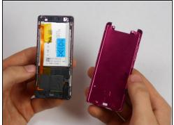
Remove the back plate from the device.
