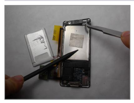
Use a nylon spudger or tweezers to remove the plastic protective plate at the top of device.
