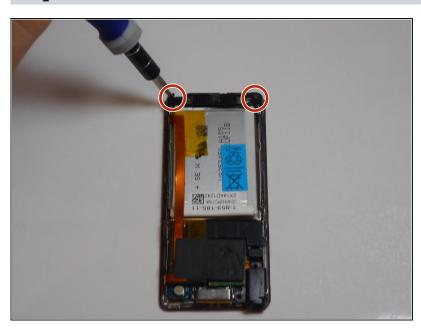
Use a Phillips #00 screwdriver to unscrew two 2 mm screws located on the top corners of the device.
